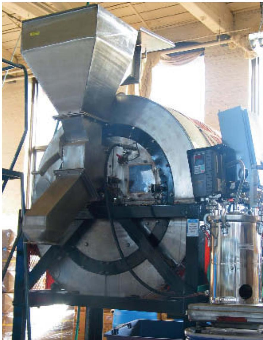
*The spraying system (lower right) sprays the liquid flavoring onto the tea leaves at 0.2 gallons per minute as the mixer’s batch vessel rotates at 3 rpm.*
