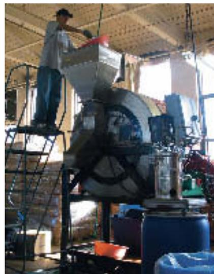
***To avoid flavor cross-contamination between batches, an operator cleans the mixer's hopper and the batch vessel's interior with water.***
