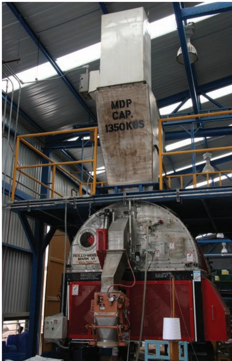
*The 3,000-pound-capacity stainless steel mixer can homogeneously blend batches as small as 5 to 10 percent of the rated capacity.*
