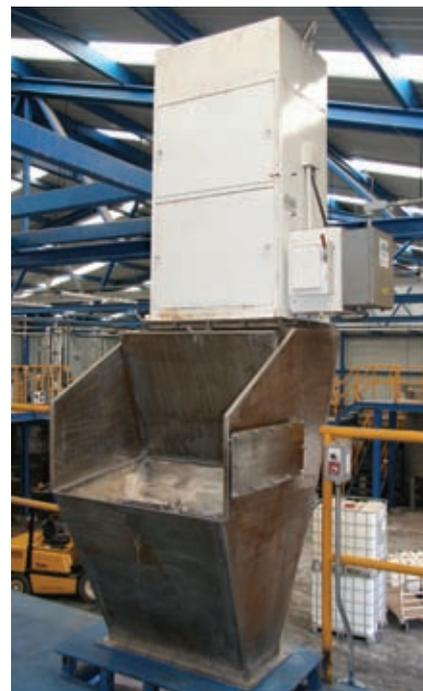
***The bag-dump station's integral dust collector pulls away dust generated when an operator manually dumps the powder ingredients into the mixer.***
