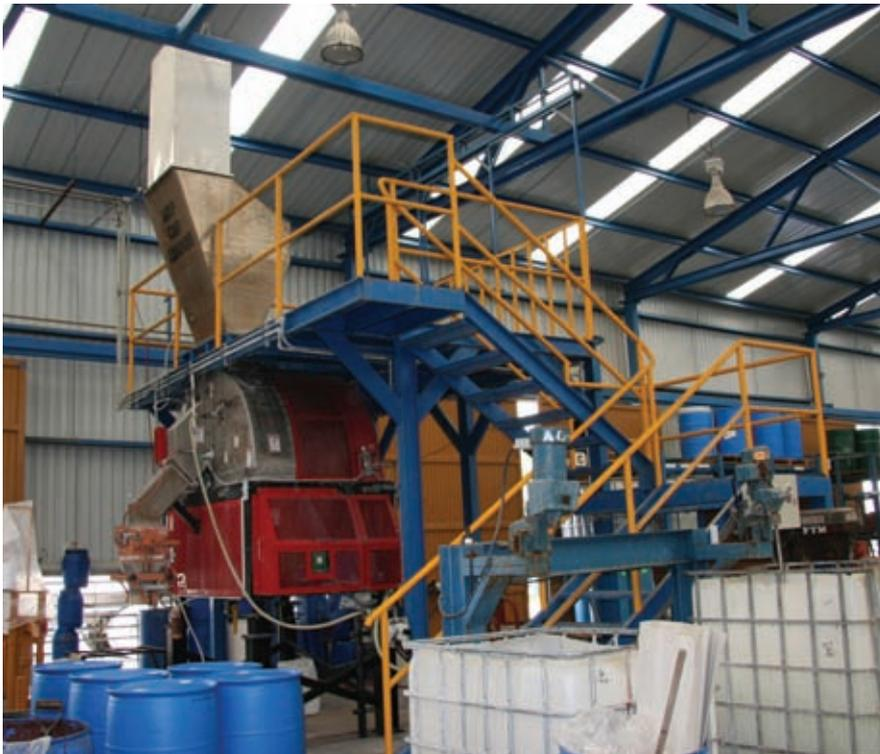
***The platform, which is built around the mixer, holds three fully loaded pallets of powder ingredients and allows an operator easy access the mixer's dust-free bag-dump station.***
