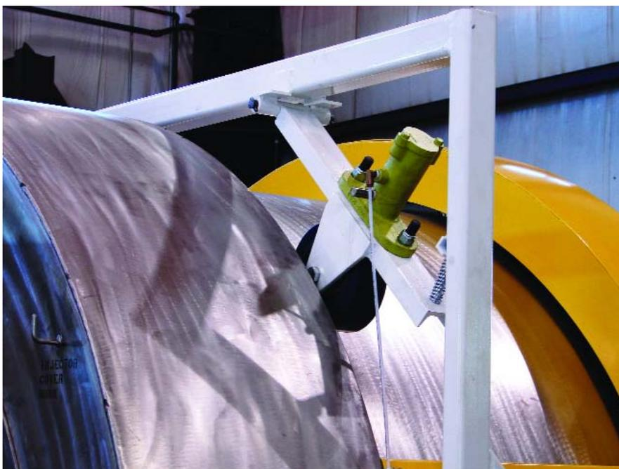
***The custom-designed mounting frame's spring keeps the wheel securely pressed against the drum's top.***
