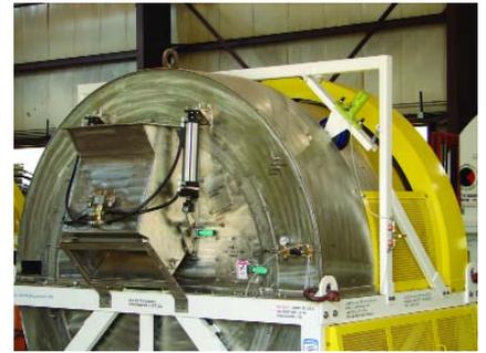
***The rolling vibrator transfers more vibration to the mixer's drum than a pneumatic piston vibrator can.***
