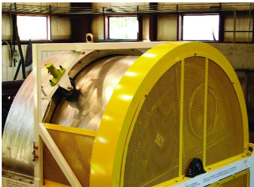
**The rolling vibrator's rubber wheel doesn't wear because it rotates with the mixing drum.**
