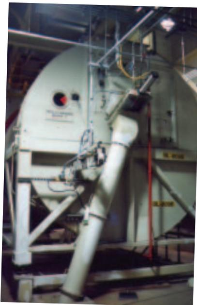
The company's mixing process required multiple steps. (1) preblend a fermented product to achieve uniform potency. (2) mix in diluents such as rice hulls and limestone, and (3) coat the particles with soybean oil to de-dust the product.
