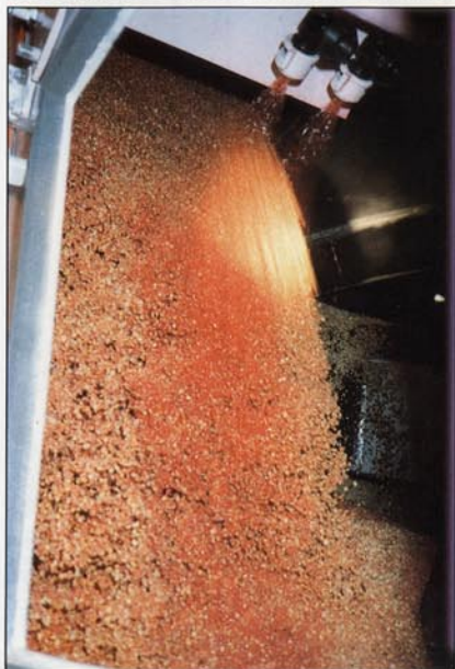
Unique free-fall impregnation coating process utilized by the Mark V "ROLLO-MIXER".
