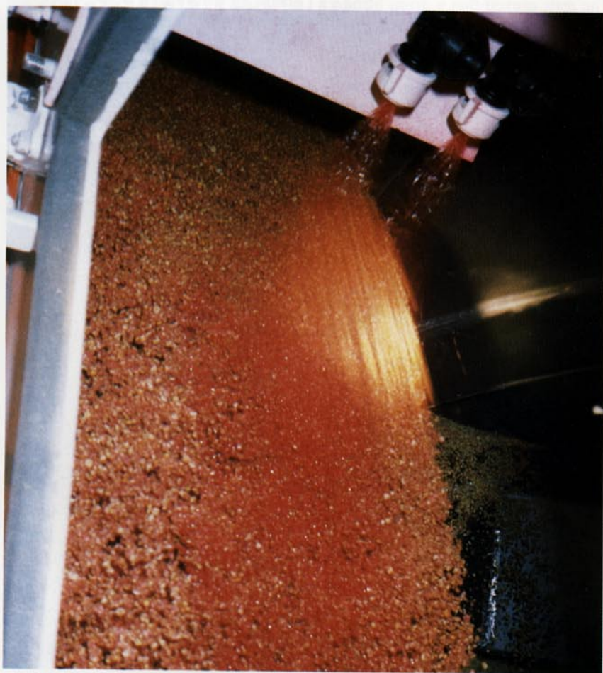
The blender's free-fall impregnation system sprays liquids onto a falling curtain of solid material, providing fast, even dispersion.
