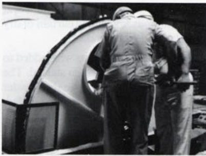
The rear access door allows the test center's staff to take samples from the blender at any time during a test.
