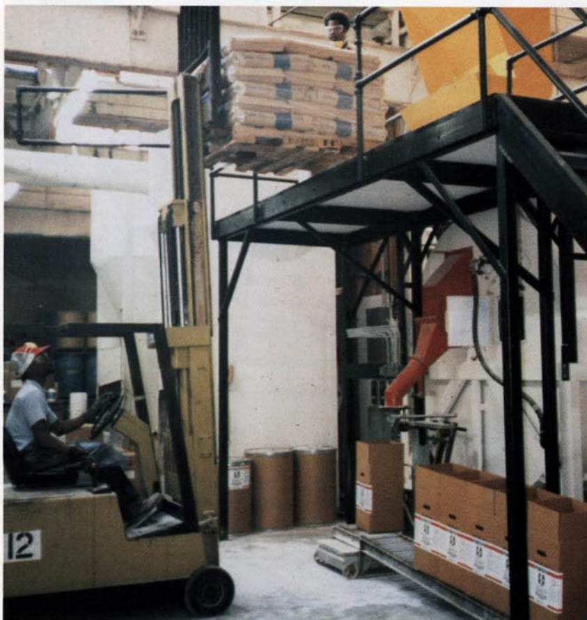
Puritan Churchill's 6,000-pound-capacity Blend/Pak system replaces four batch mixers. The system consists of a Rollo-Mixer (white unit with orange discharge spout) and a bag dump station (yellow unit) with a self-contained DCE dust collector, mounted directly above the mixer.
