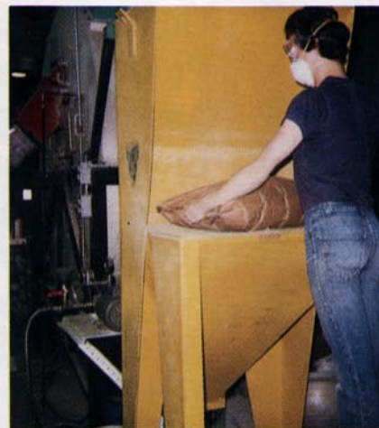
This 4 ton horizontal, rotary drum mixer and packaging system has eliminated double handling of products at Applied Biochemists, Inc.
