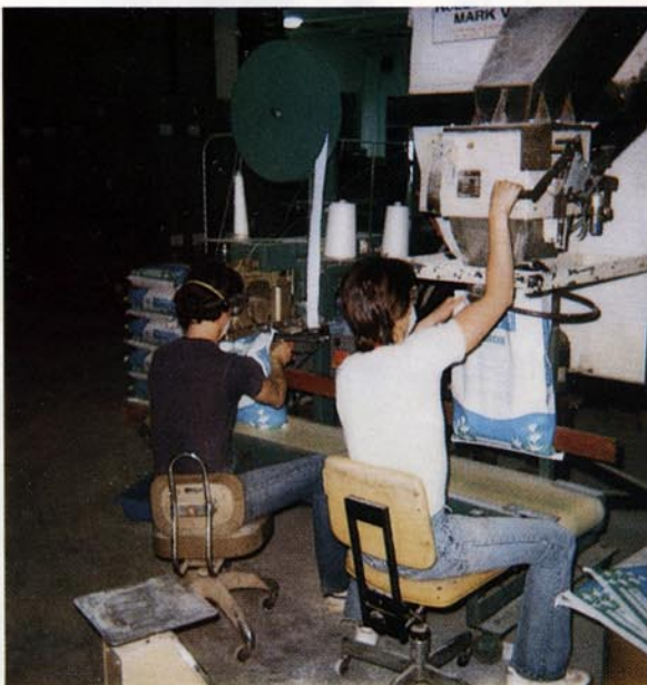
Bagger automatically stops product flow at pre-set weight. Each fill takes approximately 7 seconds
